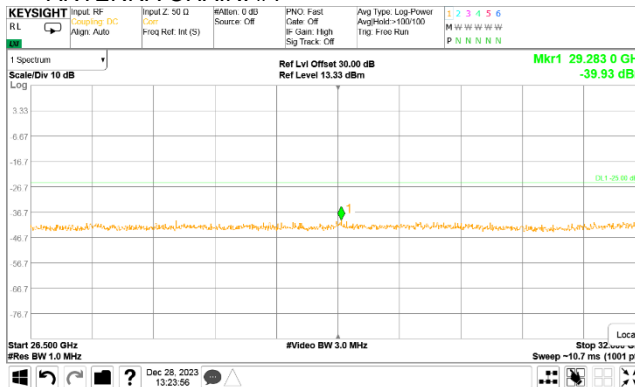
Plot 7.5.51 Spurious emission measurements in 26.5 - 32 GHz range at high carrier frequency
