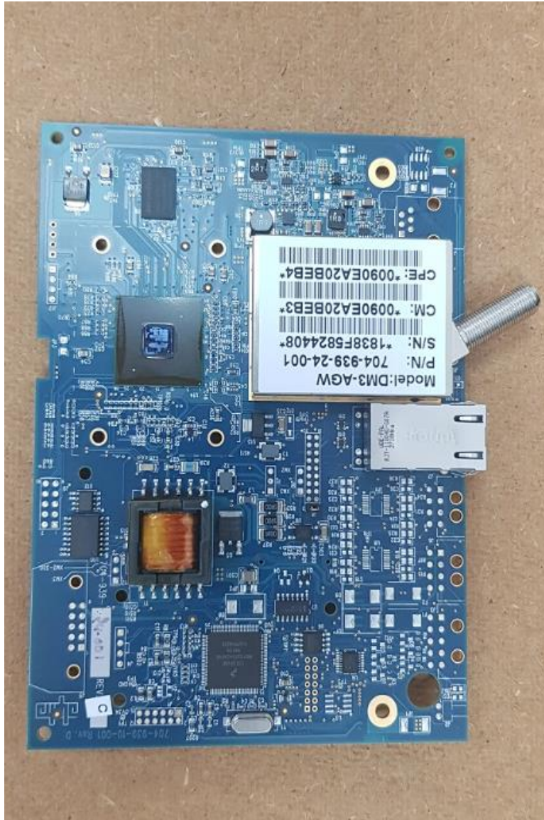
Photograph No.4 Cable Modem card_2 view
