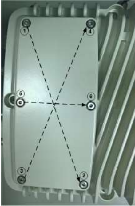
Figure 13: Screw Tightening Pattern
