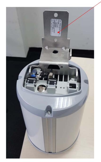
"AirSpeed1050 2.6 GHz (B41)" panel, label with FCC ID:PIDAS1050 location
