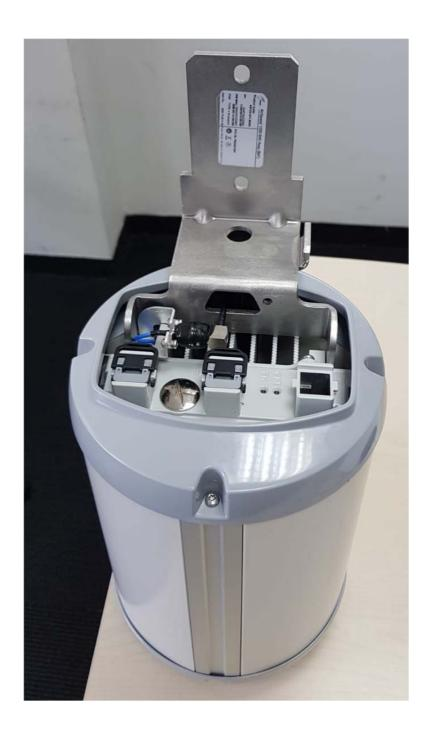
Photograph No.4 "AirSpeed1050 2.6 GHz (B41)" base station open view in plastic case
