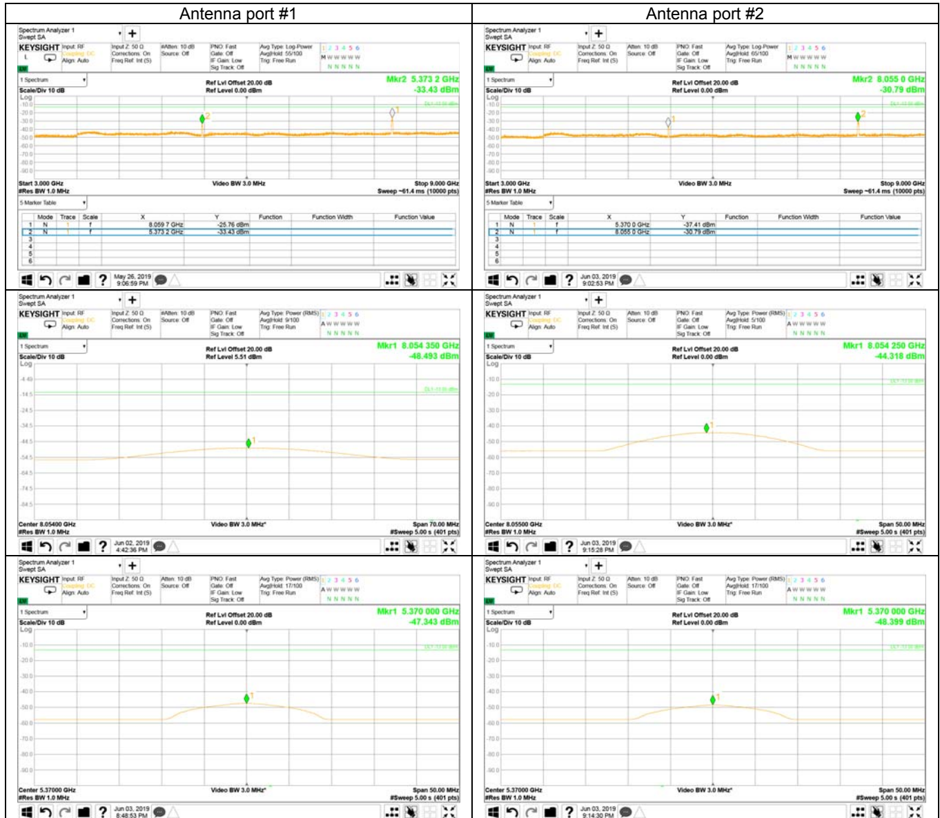
Plot 7.4.15 Spurious emission measurements in 3000 - 9000 MHz at high carrier frequency
