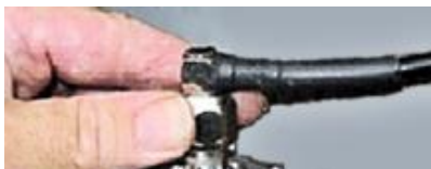
Figure 53: Connecting Antenna RF Cable
