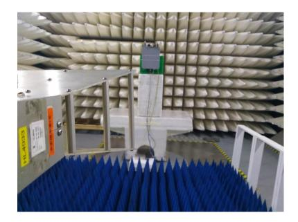
${\bf Photograph~No.5} \\ {\bf Spurious~emissions~measurement~setup~in~the~anechoic~chamber~in~18-37~GHz}$
