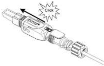
Figure 22: Holder into Transceiver
