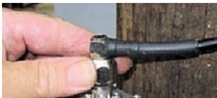
Figure 10: Connecting Antenna RF Cable
