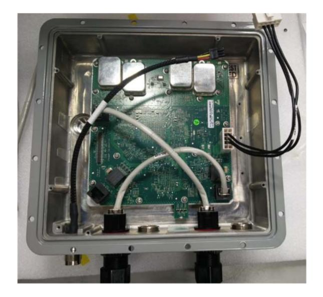
Photograph No.3 "AirSpeed 1000" base station internal view
