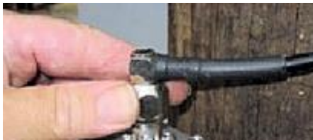
Figure 10: Connecting Antenna RF Cable
