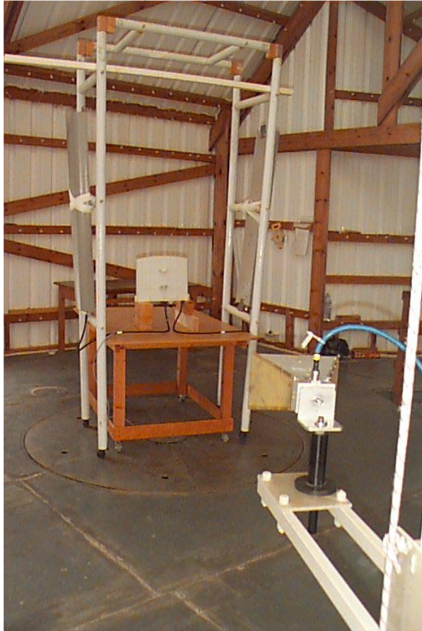
Photograph No.9 Radiated emissions measurement setup at the OATS with double ridged guide antenna, EUT with external antenna
