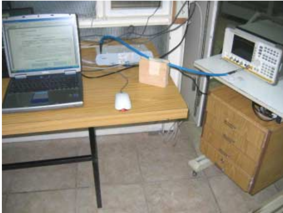
Photograph No.8 SPR peak spectral density test setup
