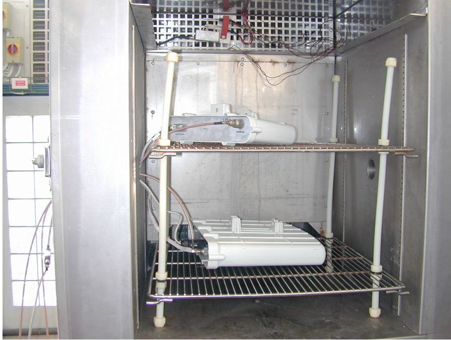
Photograph No.8 Frequency stability measurement setup
