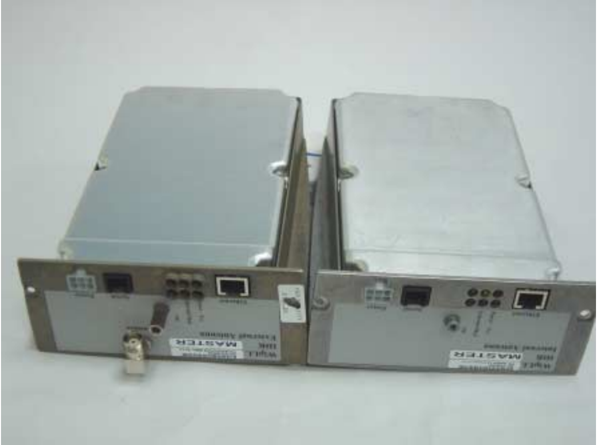
Photograph No.1 IDR 900 MHz with connector for external antenna and without connector General view
