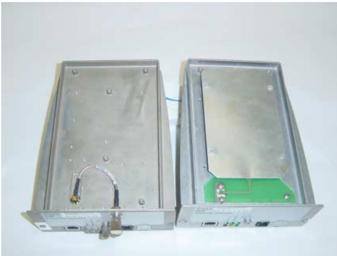
Photograph No.2 IDR 900 MHz with connector for external antenna and without connector Internal view
