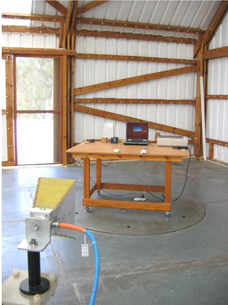
Photograph No.11 Radiated emissions measurement setup at the OATS with double ridged guide antenna, EUT with internal antenna
