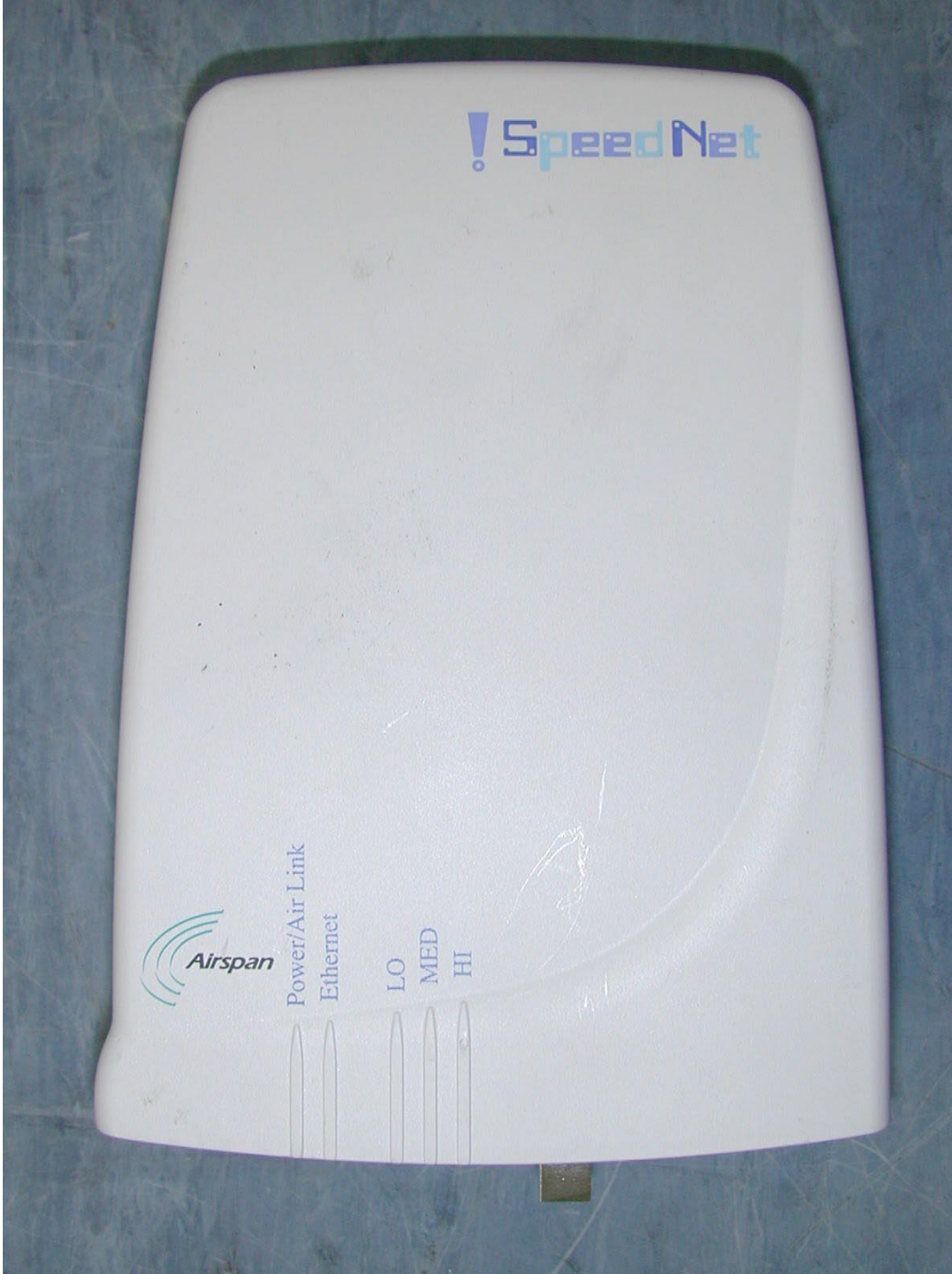
Photograph No.1 IDR 900 MHz indoor radio adapter with connector for external antenna Front view
