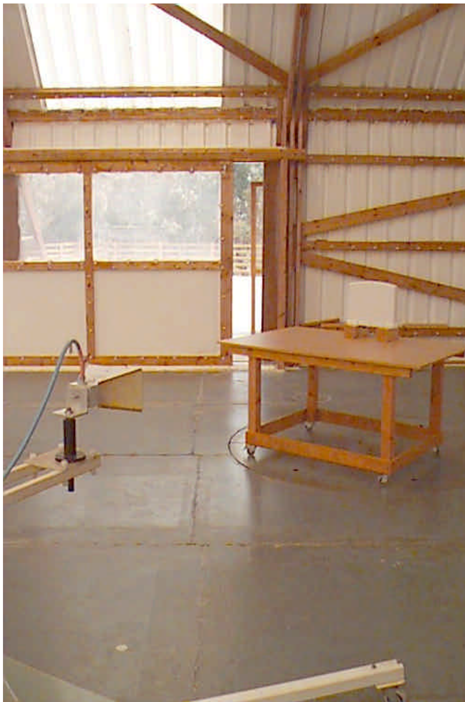
Photograph No.4 Spurious emissions measurement setup at the OATS with double ridged guide antenna
