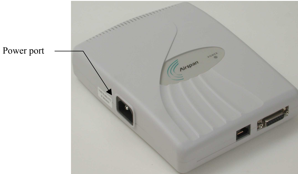
Figure 9-14: Location of SDA-1 power port
