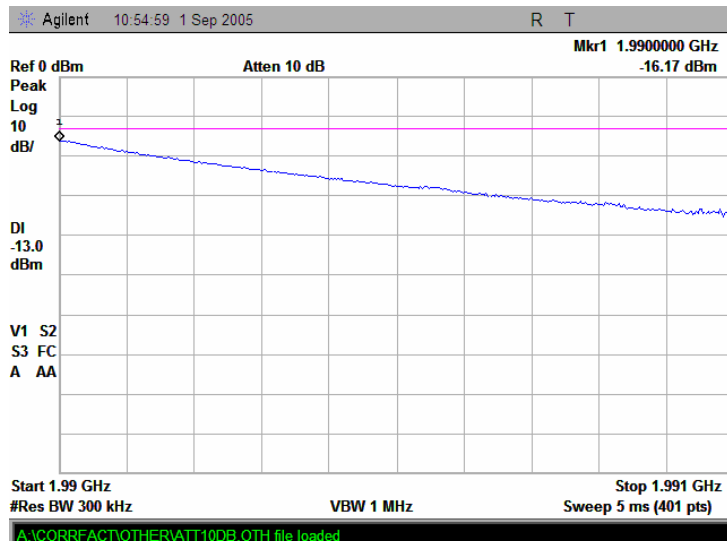
Plot 7.3.23 Spurious emission measurements in 1990 - 1991 MHz range at high carrier frequency
