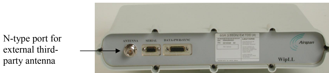
Figure 7-4: BSR model with one N-type connector
