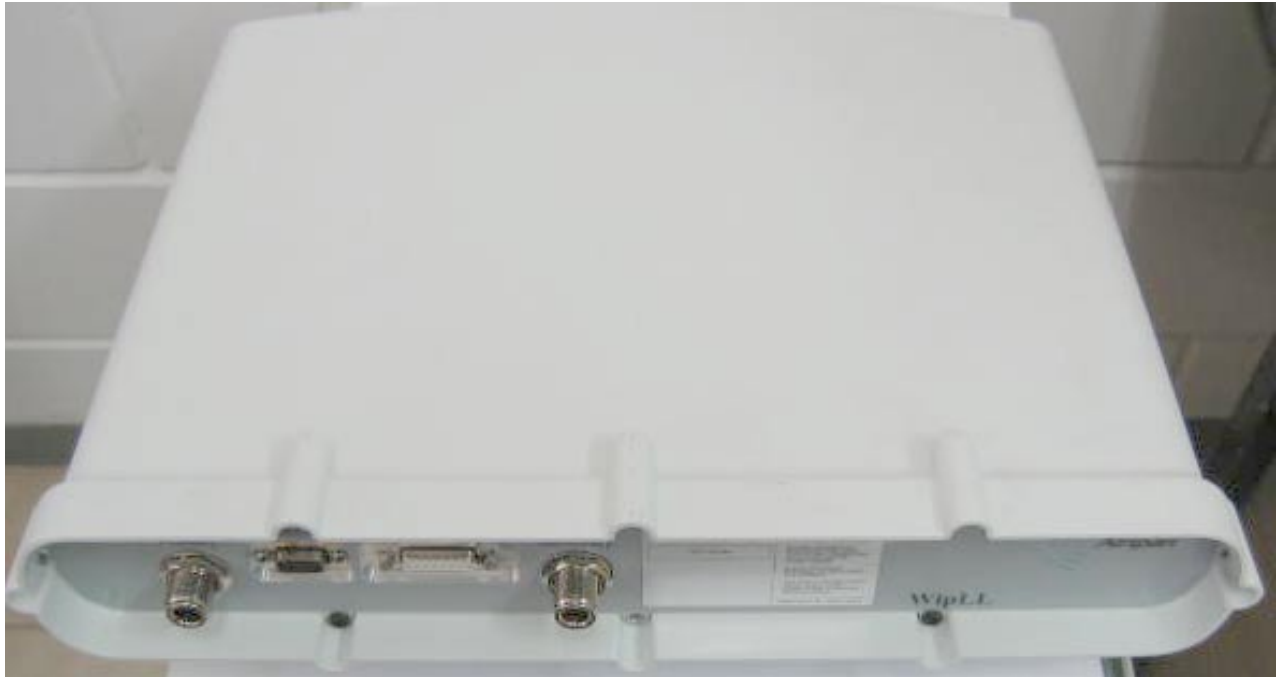
Photograph No.1 BSR 700MHz TDD Ext radio unit Front view
