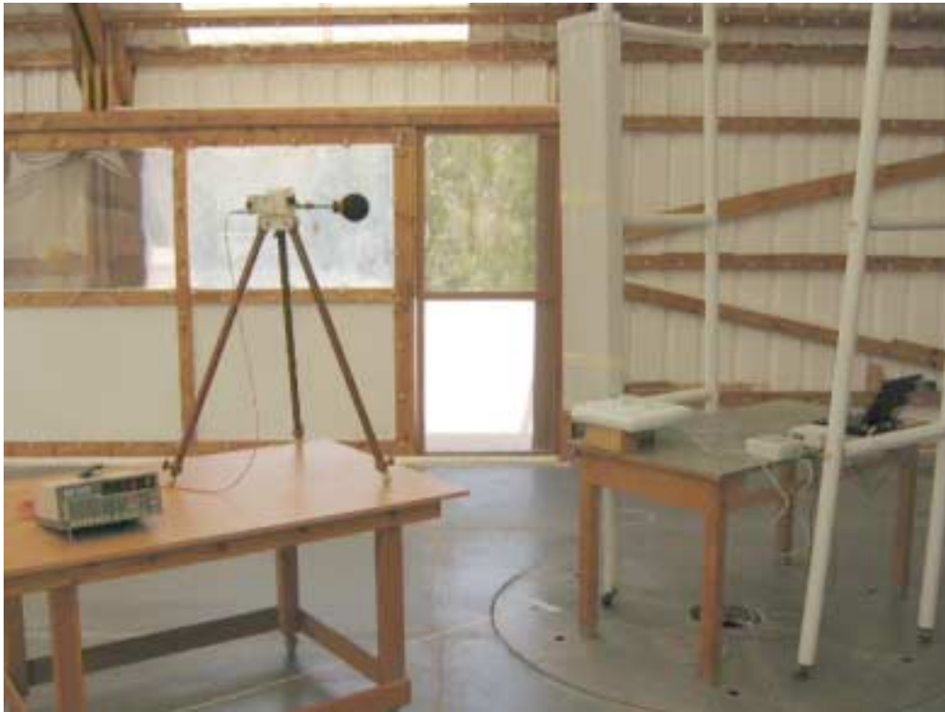
Photograph No.3 MPE measurement setup at the OATS (BSR with panel antenna, T01260801, TELSA, 14 dBi gain))
