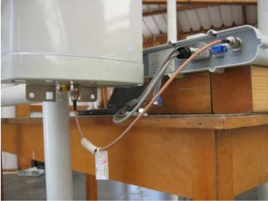
Photograph No.5 MPE measurement setup at the OATS (BSR)
