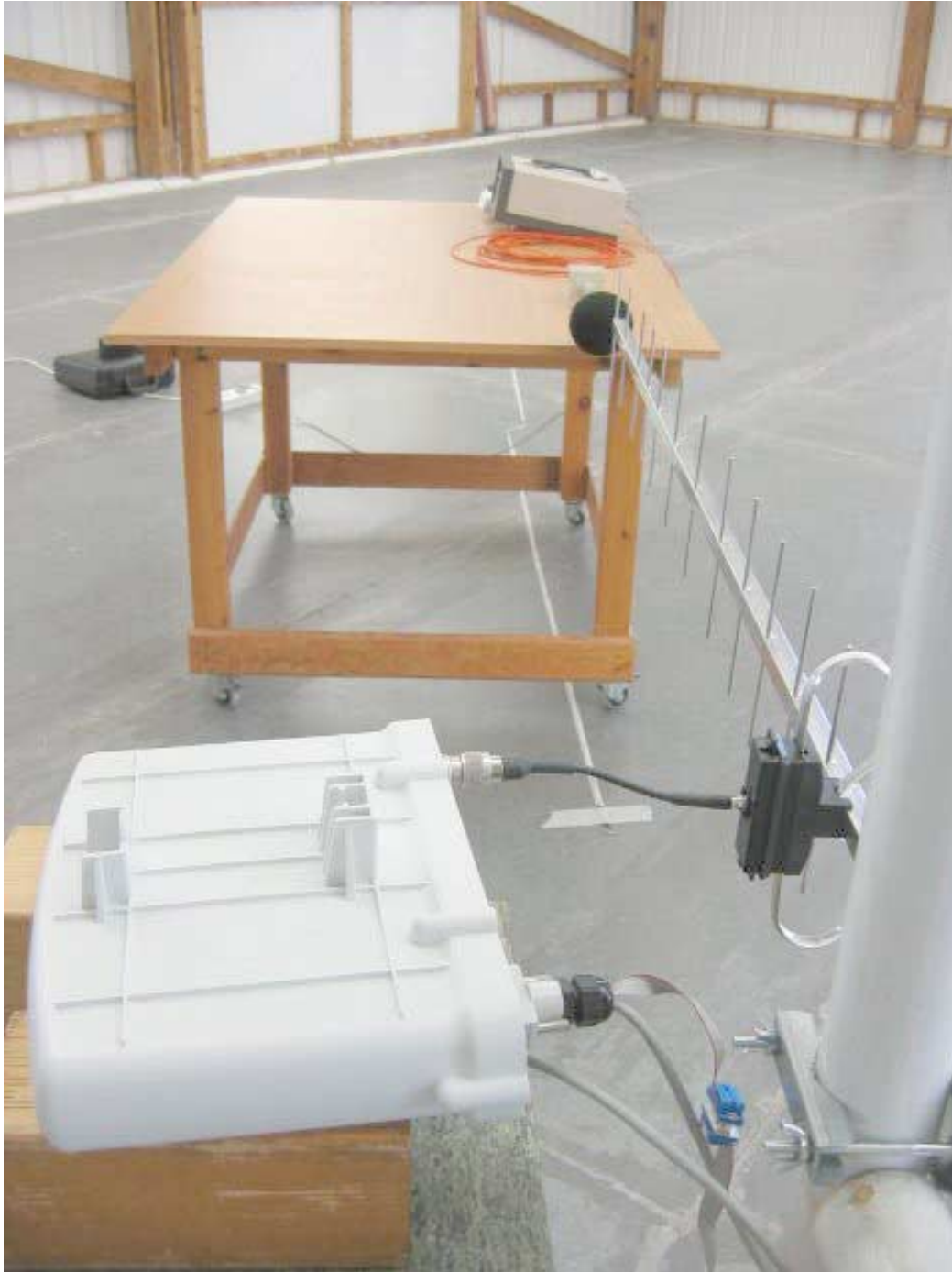
Photograph No.2 MPE measurement setup at the OATS (SPR)
