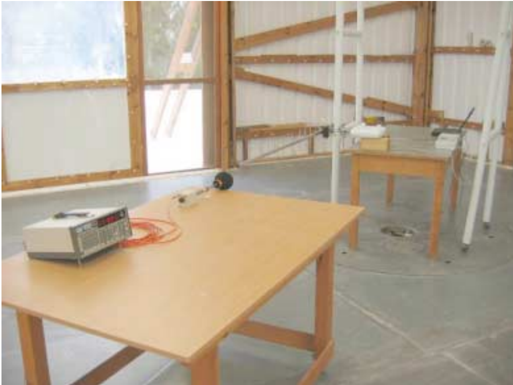
Photograph No.1 MPE measurement setup at the OATS (SPR with YAGI UF-14C antenna, 15 dBi gain)
