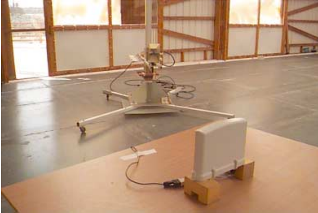
Photograph No.10 Spurious emissions measurement setup at the OATS with double ridged guide antenna, SPR
