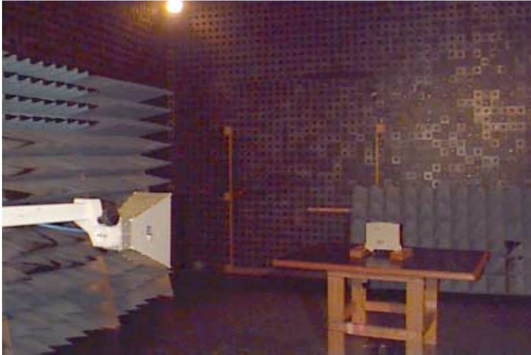
Photograph No.9 Spurious emissions measurement setup in the anechoic chamber with double ridged guide antenna, SPR
