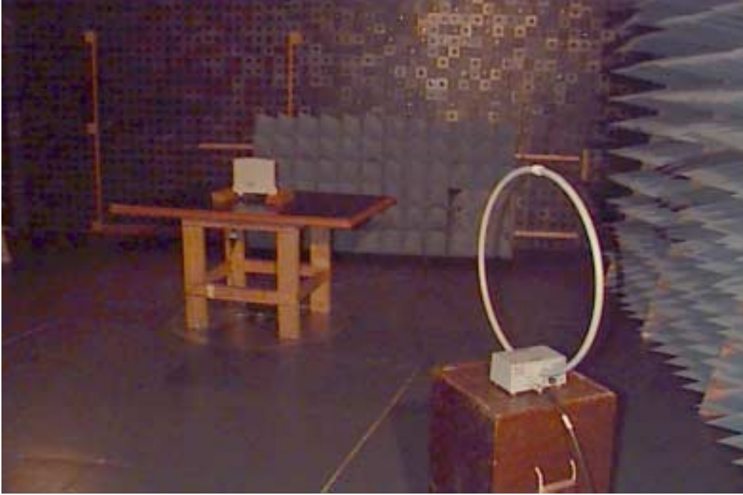
Photograph No.7 Spurious emissions measurement setup in the anechoic chamber with loop antenna, SPR
