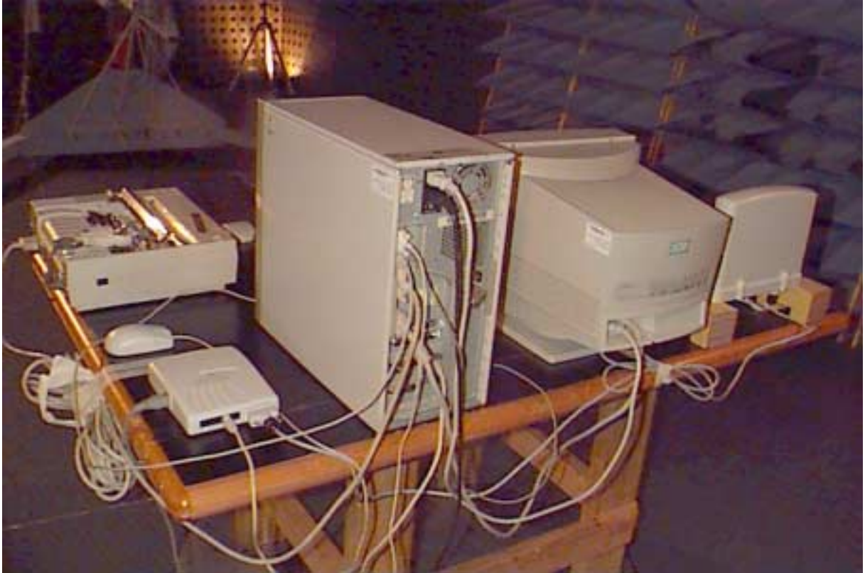
Photograph 4.8.3 Setup for radiated emission measurements, EUT view
