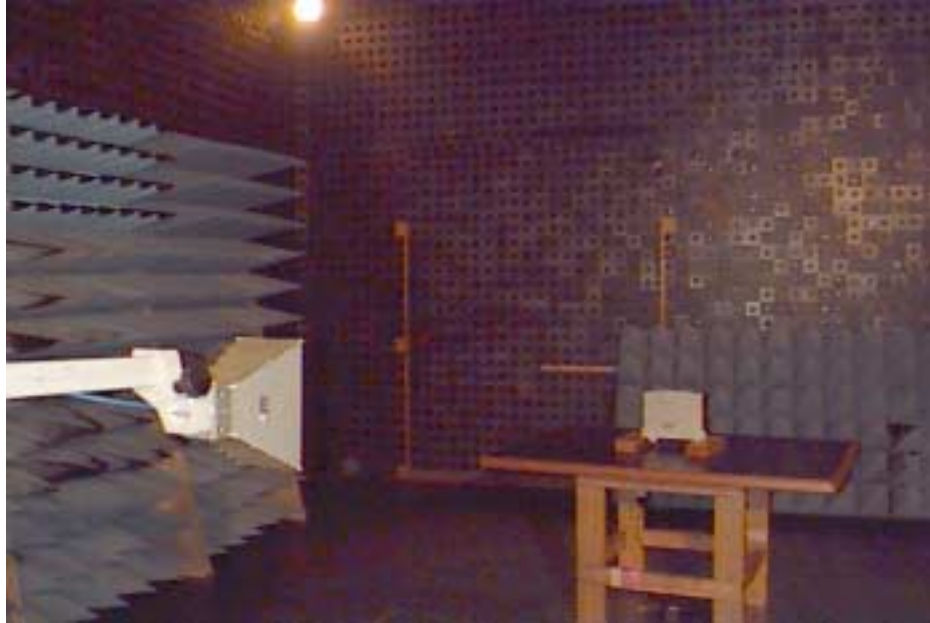
Photograph 4.5.4 Setup for spurious emission field strength measurements in 9 kHz to 6.5 GHz band, EUT view
