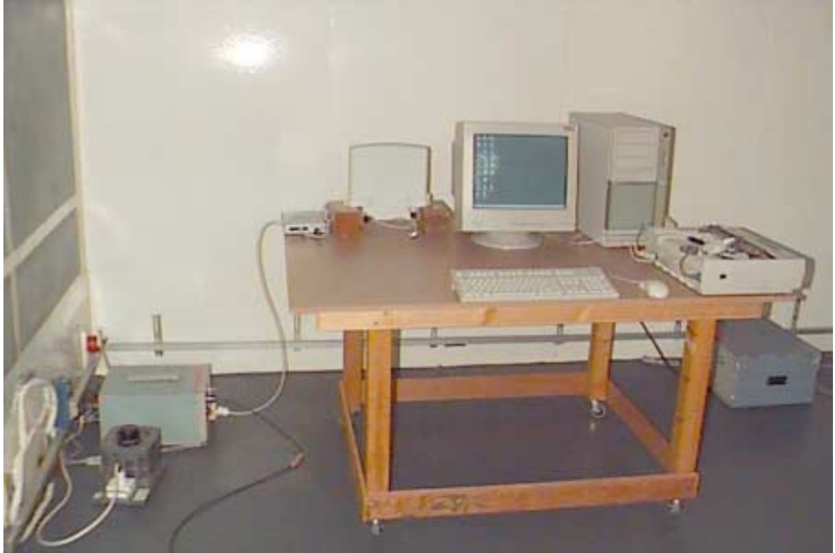
Photograph 4.6.1 Setup view for conducted emission measurements
