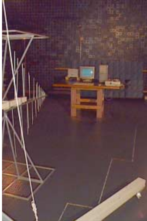
Photograph 4.8.1 Setup for radiated emission measurements in 30 – 1000 MHz range, general view
