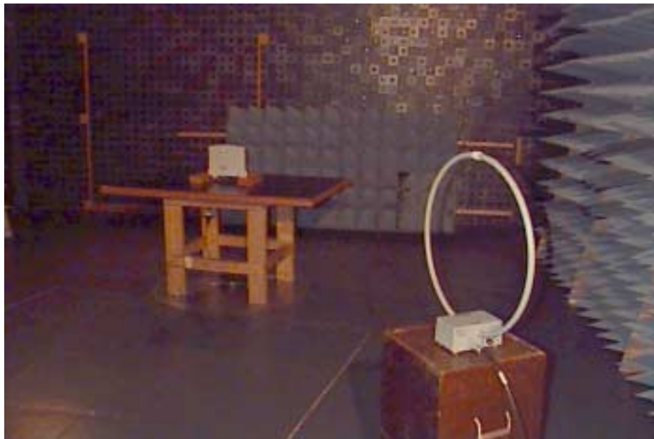
Photograph 4.5.1 Setup for spurious emission field strength measurements in 9 kHz to 30 MHz band
