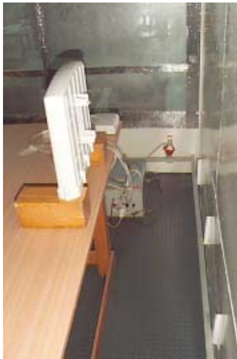
Photograph 4.6.2 Setup for conducted emission measurements, side view
