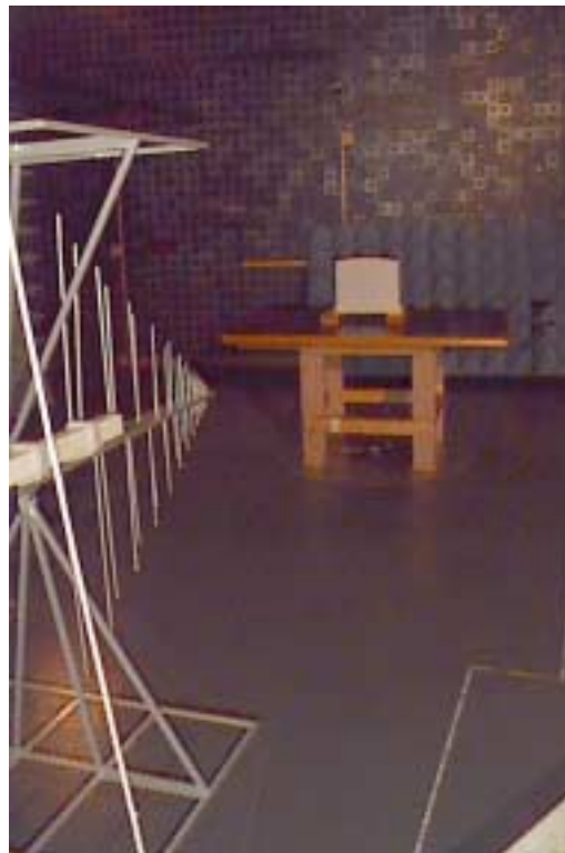
Photograph 4.5.2 Setup for spurious emission field strength measurements in 30 MHz to 1 GHz band, general view
