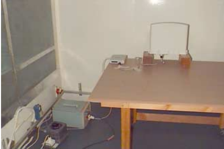
Photograph 4.6.1 Setup for conducted emission measurements, front view
