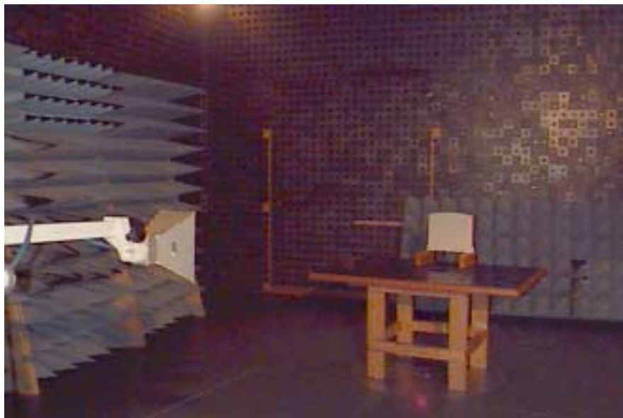
Photograph 4.8.2 Setup for radiated emission measurements in 1 – 2.2 GHz range, general view
