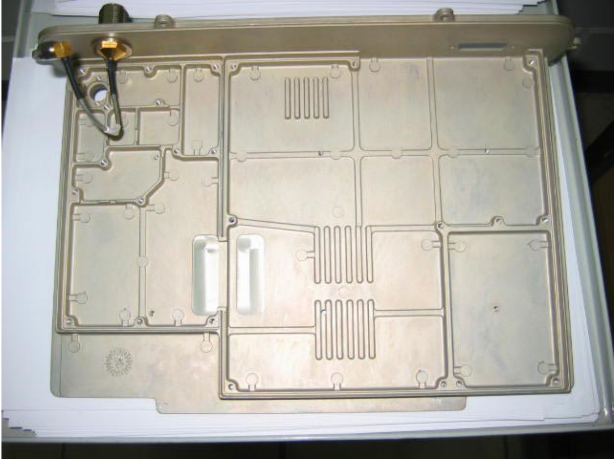
Photograph No.16 SPR 700MHz internal view
