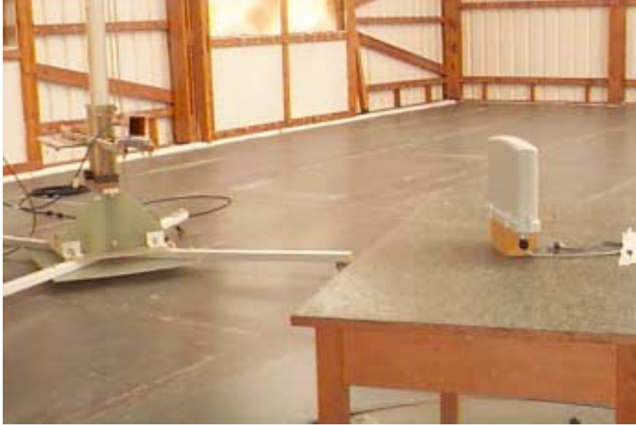
Photograph No.8 Spurious emissions measurement setup at the OATS, SPR 5.8 GHz with internal antenna
