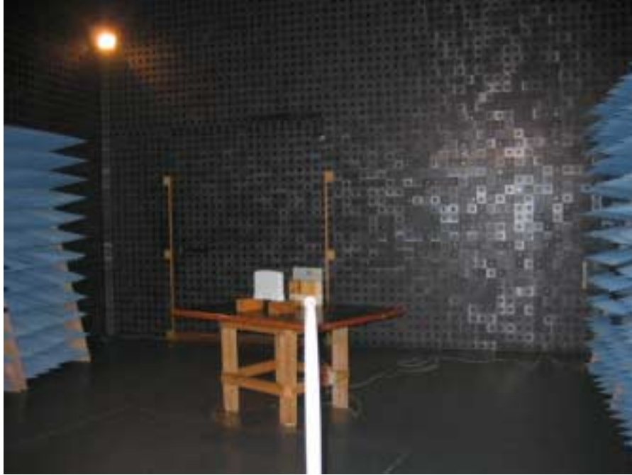
Photograph No.2 Spurious emissions measurement setup in the anechoic chamber below 30 MHz, SPR 5.8 GHz with external antenna
