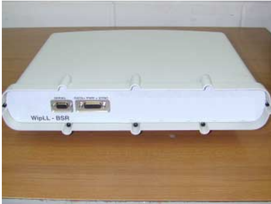
Photograph No.5 "BSR 5.8GHz TDD V-pol" radio unit General view
