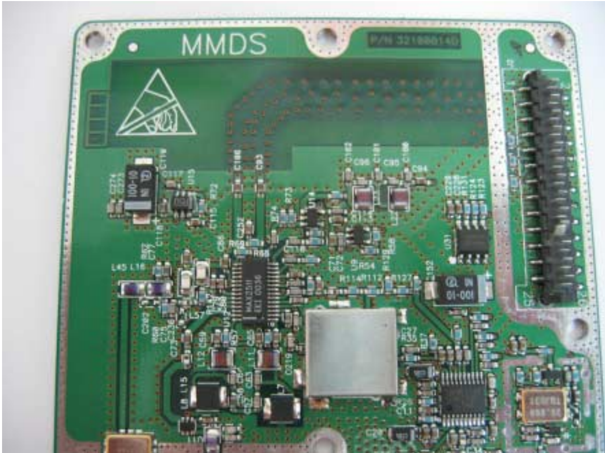
Photograph No.5 BSR 2.5GHz, RF module close front view
