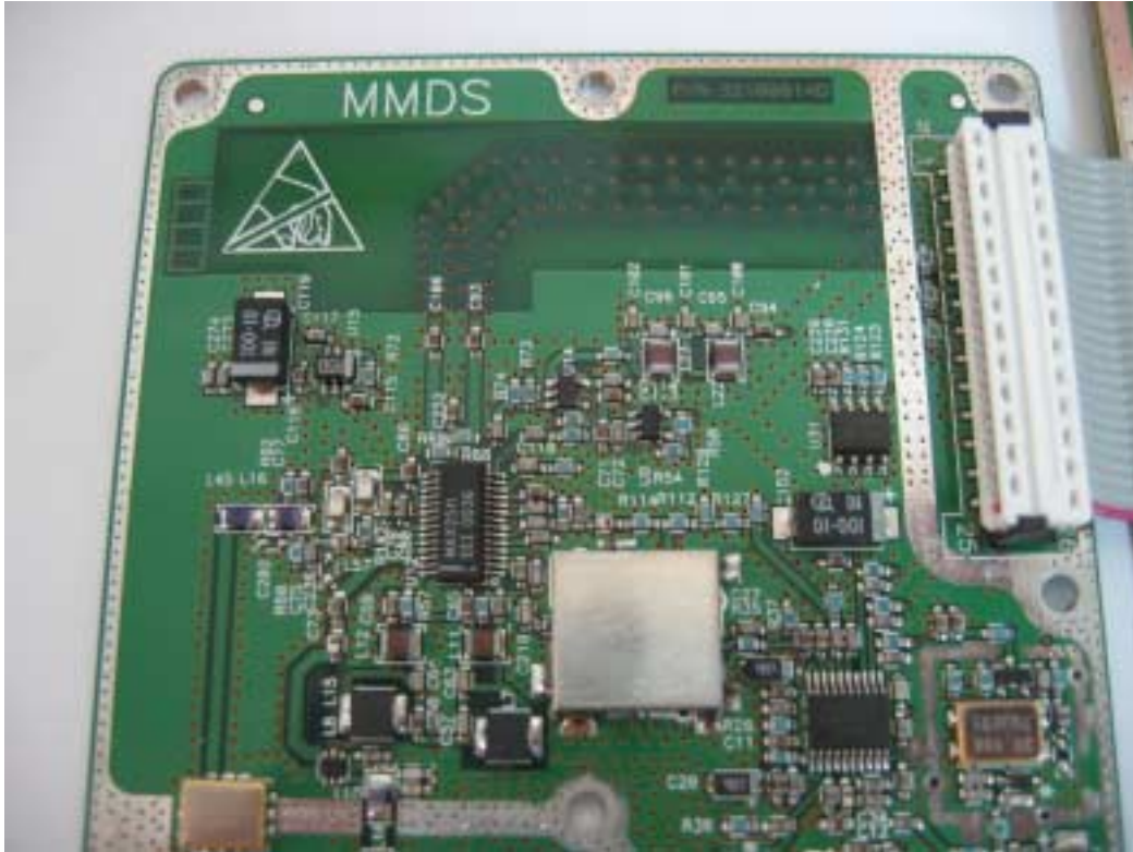
Photograph No.15 SPR 2.5GHz TDD V-pol RF module close view
