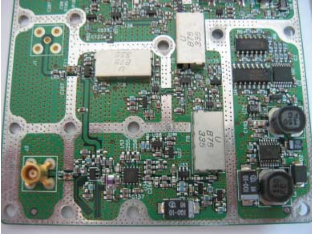
Photograph No.17 SPR 2.5GHz TDD V-pol RF module close view
