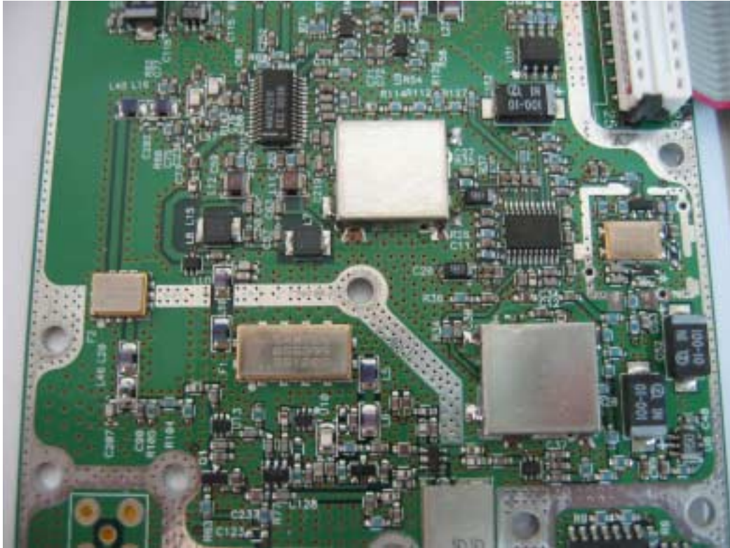
Photograph No.16 SPR 2.5GHz TDD V-pol RF module close view
