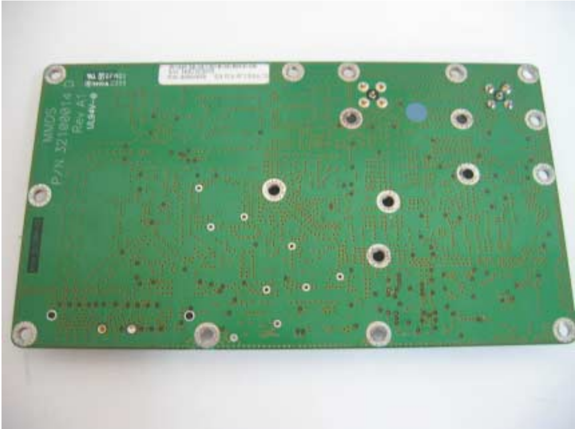
Photograph No.8 BSR 2.5GHz, RF module second side view
