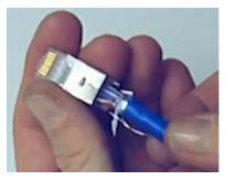
11. Push the wires all the way into the RJ45 connector until the front of the wires butt against the front of the connector (inside). Visually inspect to verify that the wires are fully inserted.
