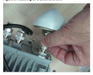
Caution: Take care not to over tighten so as not to damage the threads.
