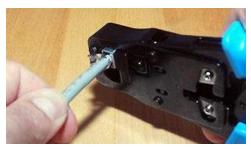
Note: All pins should be fully compressed and of equal height after crimping.
