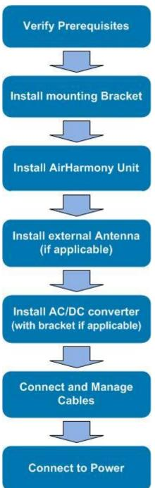
Caution: Antennas must be connected and attached before AirHarmony-1000 is powered on.
