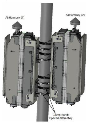
The difference in height between the installed units after installation will be 40mm.
