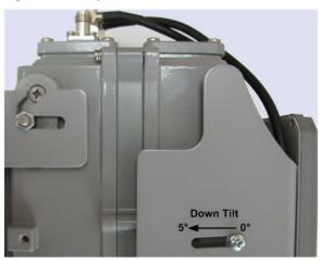
After adjusting to the required tilt amount tighten both flange nuts and both screws. The antenna has an electrical fixed down-tilt of 1°.
