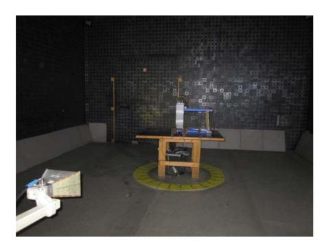
$\label{eq:Photograph No.8} Photograph No.8 \\ Spurious emissions measurement setup in the anechoic chamber in 18 – 27 GHz$
