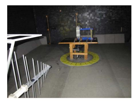
$\label{eq:Photograph No.7} Photograph No.7 Spurious emissions measurement setup in the anechoic chamber in 1 – 18 GHz$
