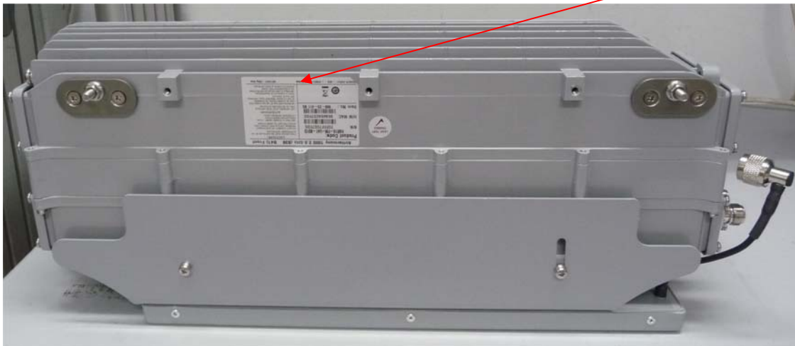
“AirHarmony 1000 2.5 GHz (B38, B41)”side panel, label with FCC ID:PIDAHR2500 location
