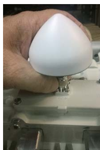
Figure 6: Attaching GPS antenna to unit
