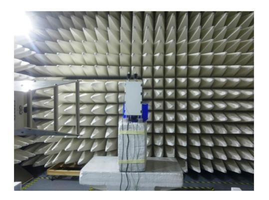
$\label{eq:Photograph No.7} Photograph No.7 Spurious emissions measurement setup in the anechoic chamber in 18 – 37 GHz$
