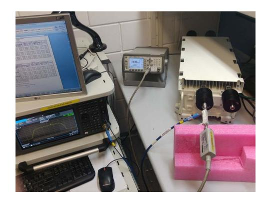
Photograph No.3 Conducted spurious emissions emission mask and OBW measurement setup
