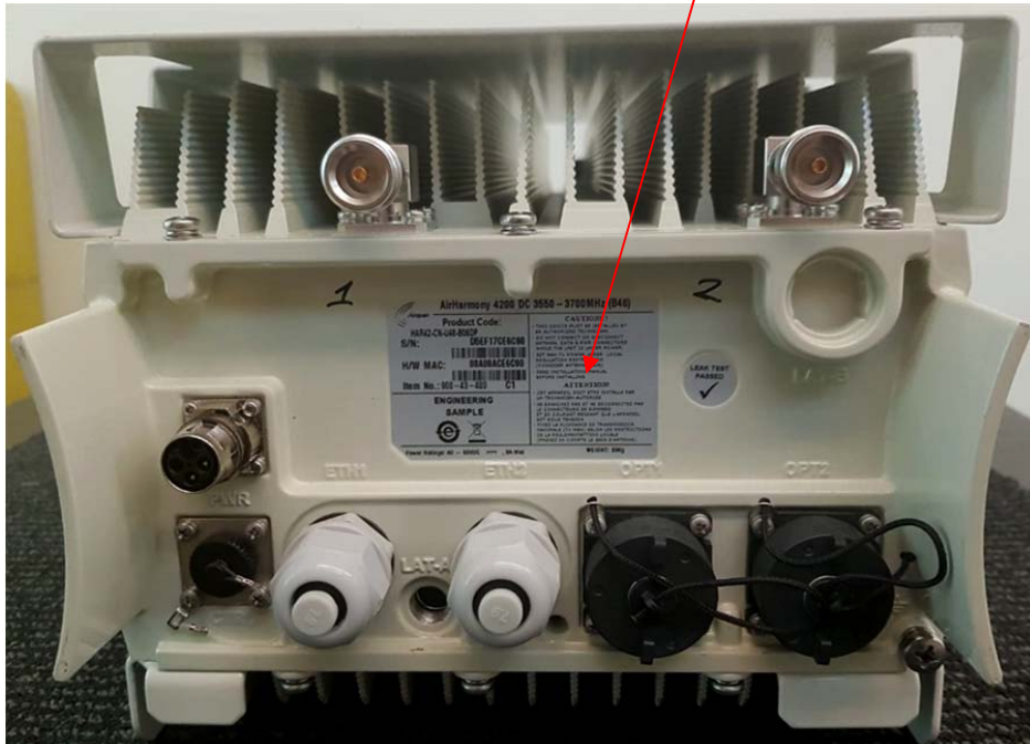
“AirHarmony 4200 3550-3700MHz (B48)” side panel, label with FCC ID:PIDAH4200A location
