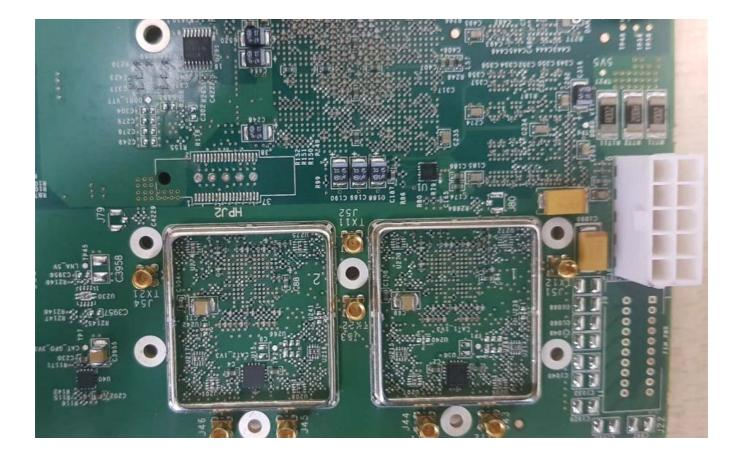
Photograph No.4 RF PCB close view with shields removed
