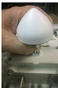
Figure 6: Attaching GPS antenna to unit
