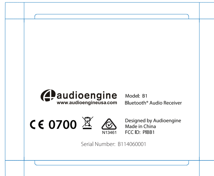
B1 case bottom art - REV09 Serial Number Format year / month / serial number 13 01 0001
