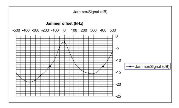
Disregarding the data points at -450 kHz, -400 kHz, -350 kHz, and -300 kHz, the worst data point is found to be at -16.6 dB (at -250 kHz). Thus, the PG becomes
