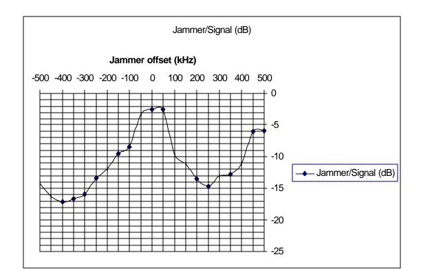
Disregarding the data points at ~450 kHz, ~400 kHz, ~350 kHz, and ~300 kHz, the worst data point is found to be at -14.7 dB (at +250 kHz). Thus, the PG becomes
