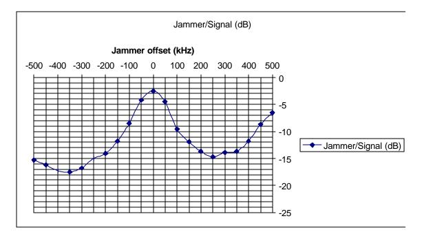
Disregarding the data points at -450 kHz, -400 kHz, -350 kHz, and -300 kHz, the worst data point is found to be at -15.3 dB (at -500 kHz). Thus, the PG becomes
