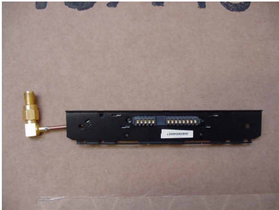
Picture 4 : Portofino with temporary antenna connector and without tripod bottom side
