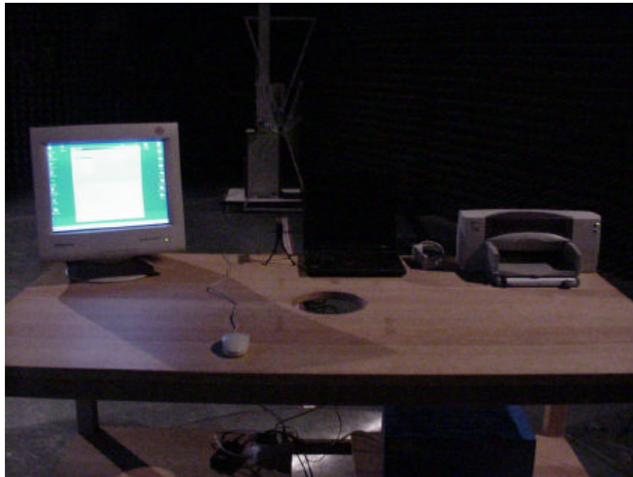
Picture 1 : Setup for radiated emission measurement
