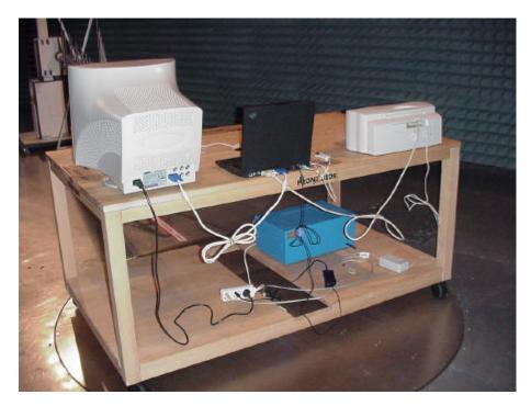
Picture 2 : Setup for radiated emission test below 1 GHz, rear view
