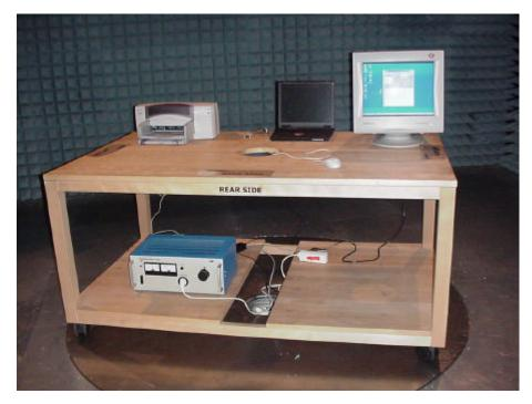
Picture 1 : Setup for radiated emission tests below 1 GHz
