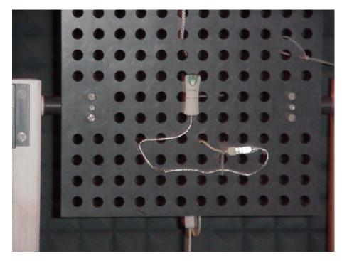
Picture 4 : Setup for radiated emission tests above 1 GHz
