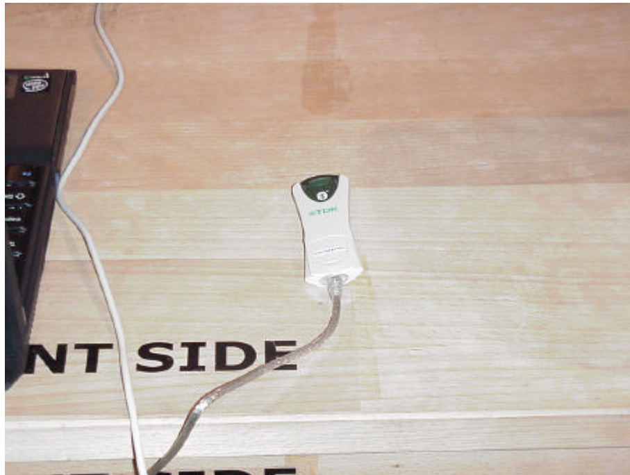
Picture 3 : Setup for radiated emission test below 1GHz, detailed view
