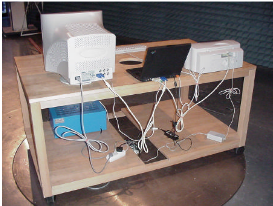
Picture 4 : Setup for radiated emission tests below 1 GHz, rear view
