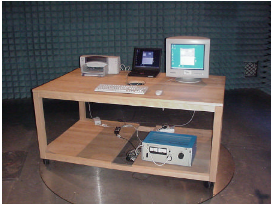
Picture 3 : Setup for radiated emission tests below 1 GHz
