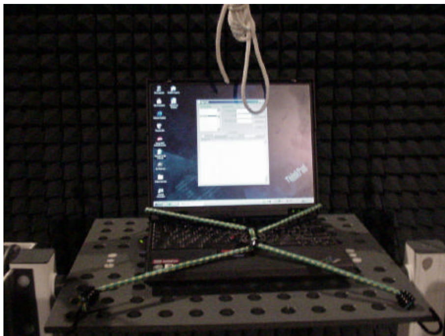
Picture 2 : Setup for radiated emission tests above 1 GHz
