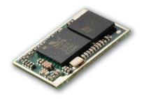
The BTM510 and BTM511 are low-power Bluetooth® modules designed for adding robust audio and voice capabilities. Based on the market-leading Cambridge Silicon Radio BC05 chipset, these modules provide exceptionally low power consumption with outstanding range. Supporting the latest Bluetooth® Version 2.1+EDR specification, these modules provide the important advantage of secure simple pairing that improves security and enhances easy use.
