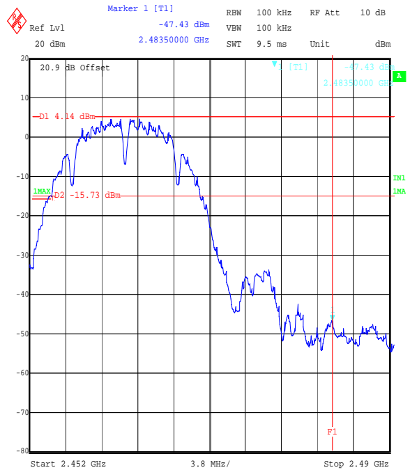
Title: EZURIO 2.4 GHz WLAN Module. FCC Part 15.247 Cond. BandEdge Comment A: 48271JD05 Top Channel DSSS BPSK Date: 8.SEP.2006 16:27:16
