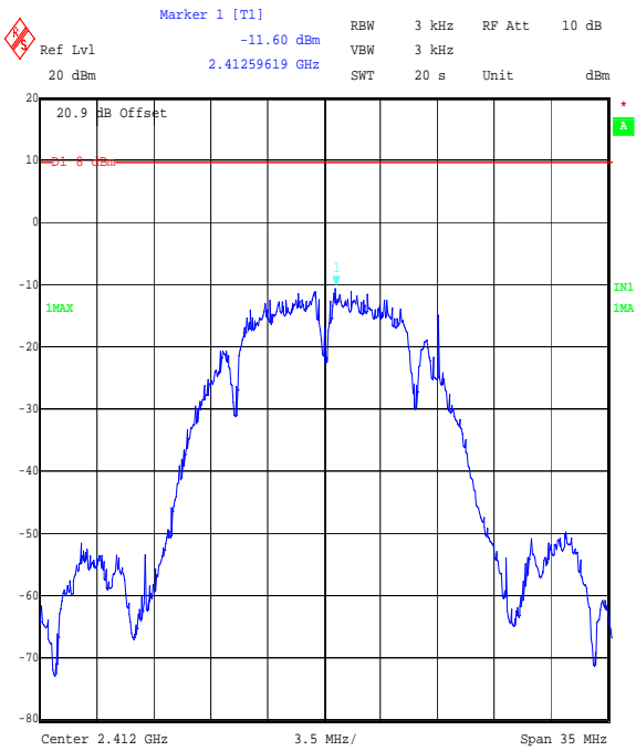
Title: Ezurio 2.4 GHz WLAN module, FCC P15.247 Spectral Density Comment A: 48271JD05 Bottom Channel, BPSK DSSS. Date: 5.SEP.2006 14:10:12
