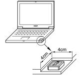
The directivity is measured using a mockup of A4-sized notebook computer with a built-in antenna. The mockup is made of copper plate which scatters electric wave from the antenna. Open a 4×4cm window and install the antenna mounted on TDK STD evaluation base.
